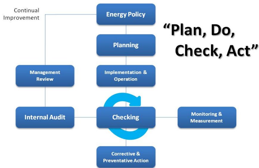
Figure 1 Energy Management System Model
